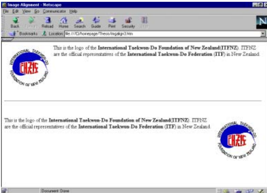
Figure 8.7 Using the LEFT and RIGHT values of ALIGN to create floating images. Notice how the text continues to wrap around the image, unlike the example in Figure 8.6.
